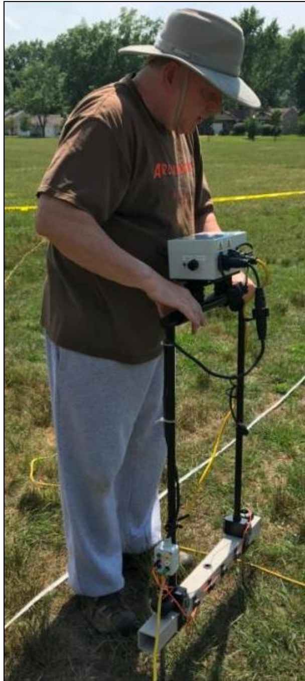
Figure 14: Student employing the RM-15D electrical resistance meter. The mobile array shown here has two metal probes inserted into the ground. One probe forms part of a pair of probes (the other is approximately 25m away, not shown) that generate a subsurface electrical field. The other probe (and its partner also 25m away) measures the resistance locally to the flow of electricity.
